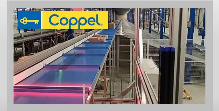
Support and maintenance of high-performance automatic system. Double-deck tray sorter with side channels, capable of a maximum capacity of more than 20,000 puts per hour.
