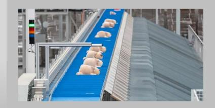
Motorized and gravity conveyors carry the merchandise throughout the Distribution Center efficiently.
