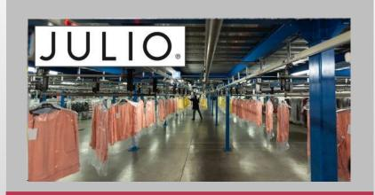
An ideal overhead conveyor system to process and store, with very high efficiency, hanging, and flat garments.
